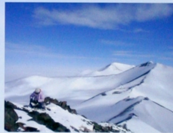
Figure 2. Sampling in the Eternity Range. Geological samples were collected across Mount Faith, Mount Sullivan and Engel Peaks. The "dip-stick" sampling approach was adopted to measure the maximum ice extent and thinning rates of the ice sheet. A total of 39 samples were taken for cosmogenic isotope analysis. This poster shows the results for the 5 highest altitudinal samples only.
