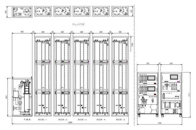
Figure 1: Schematic view of pCO<sub>2</sub> controlled seawater preparation system (AICAL system).
