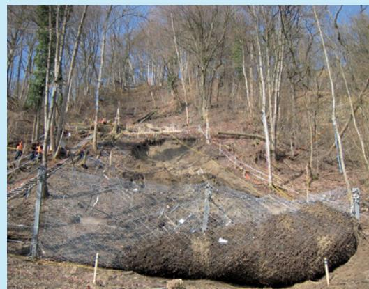
Artificial land slide triggered as part of the TRAMM project.
