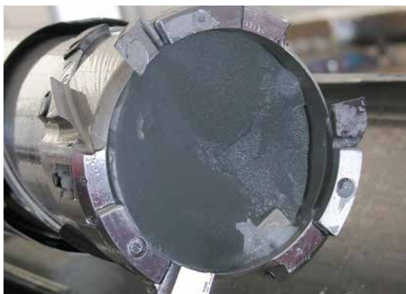
Drill head of the EPICA drill used at Dome C (Antarctic) containing a 10 cm diameter ice core © Jakob Schwander, University of Bern
