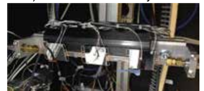
Thermal Figure of Merit characterisation measurement on a 3-celled barrel staff sample using \text{CO}_2 cooling.
