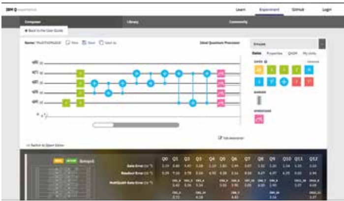
Figure 4: The "IBM Q experience" web interface gives access to experimental quantum processors with 5 and 16 qubits for exploring basic quantum circuits. (see https://www.ibm-research.com/ibm-qx )
