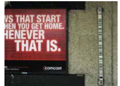
Figure 4: Boston, Subway station: The barcode rod is recorded by a digital level instrument, and mechanical deformations of sub-mm amplitude are quantitatively detected.
