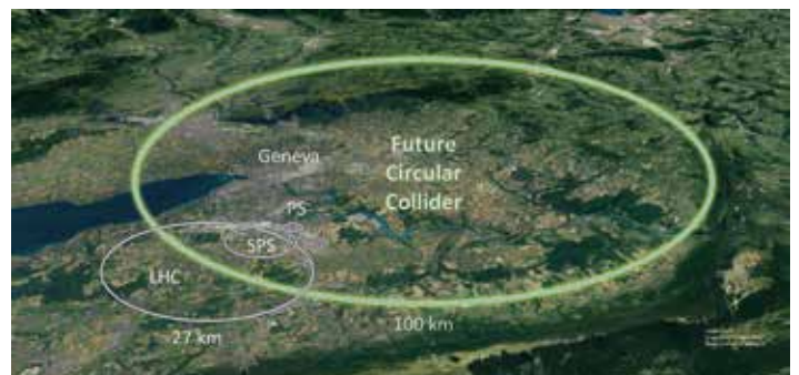
Aerial view showing the current ring of the LHC (27 km) and the proposed new 100 km tunnel that could host different colliders modes (FCC-ee, FCC-hh, FCC-he). Picture: © CERN
