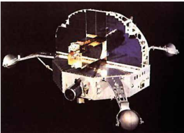
Fig. 1 – NASA's Orbiting Observatory OSO-6. The spacecraft consisted of a rotating 'wheel' providing gyroscopic stability and a 'sail' that contained solar cells for electricity generation and also held two pointed instruments. During the daylight portion of the orbit 7 an electric motor drove the 'sail' relative to the 'wheel' and kept the solar cells in sunlight. By slightly varying its speed, that same motor could also induce an azimuthal scan of two pointed instruments. Together with a second motor that controlled the elevation, one could command the telescope axes of the pointed instruments to perform a raster pattern 8 and thus to cover an extended field of view. 9 (Image: Ball Brothers Research Corporation.)
