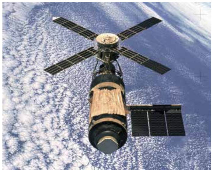
Fig. 6 – The Skylab space station, consisting of an ‘Orbital Workshop’ (visible below the yellow ‘parasol’), which provided living and working space for the astronauts, and of the Apollo Telescope Mount (ATM). The front ends of the eight solar telescopes in the ATM can be seen inside the white rim framed by four solar panels. Joint daily observing programmes for all instruments were devised on the ground by a group of solar physicists representing all the investigator groups and were then transmitted to the astronauts on Skylab for execution – with the proviso that unexpected behaviour of the Sun might lead to improvised changes to be decided by the astronaut-observer on duty. The ‘parasol’ covering the ‘orbital workshop’ had to be installed by the first crew arriving at Skylab, because the so-called micro-meteorite shield of the workshop, which also would have provided thermal insulation, was lost during the launch of Skylab and also led to the loss of what would have been an additional solar panel on the left side of the orbital workshop. (Image taken by the third Skylab crew, Credit: NASA.)
