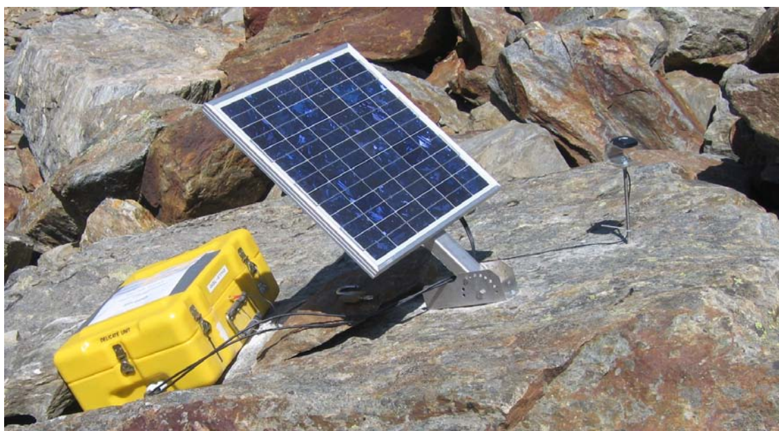
Figure 1. GPS station installed on the rock glacier, including (from right to left) GPS antenna, solar panel and instrument box containing GPS receiver and battery.
