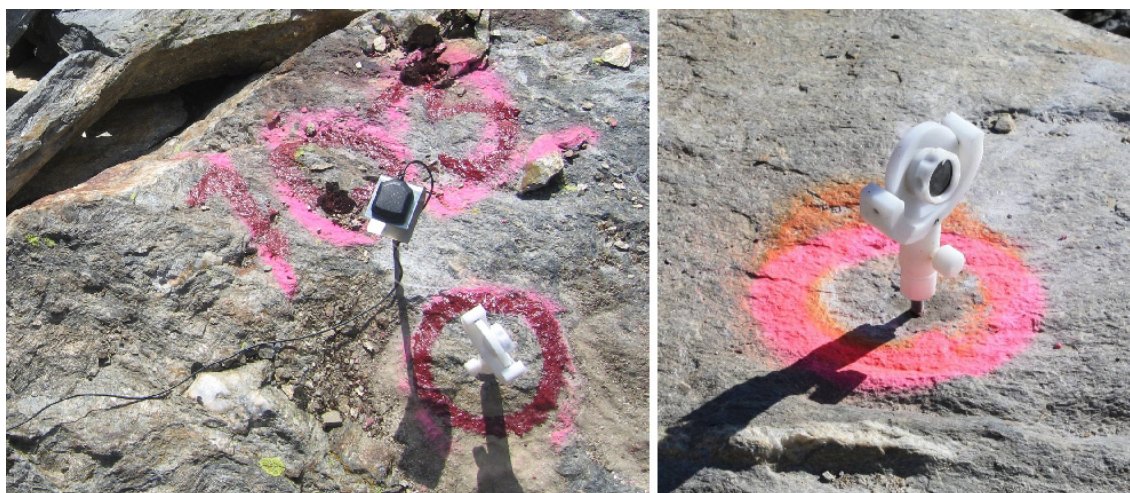
Figure 2. GPS antenna and mini prism installed on the same boulder (left picture) and mini prism in detail (right picture).
