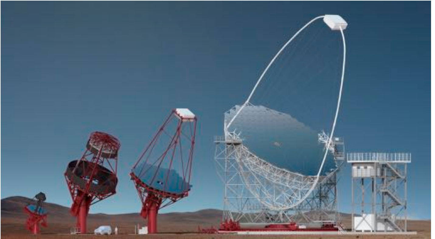
Fig. 1: The four telescope designs of CTAO, from left to right: the two innovative Schwarzschild-Couder telescopes, the Small Sized Telescope (SST) with 4 m diameter equivalent mirror surface and the about 12 m Telescope (SCT); the Davies-Cotton Middle Sized Telescope (MST) of about 12 m diameter optical system and the Large Sized Telescope (LST) with 23 m diameter parabolic reflecting surface. The SSTs, MSTs and LSTs will be deployed for the Alpha-configuration of CTAO, currently in construction (Credit: Gabriel Pérez Diaz, IAC)
