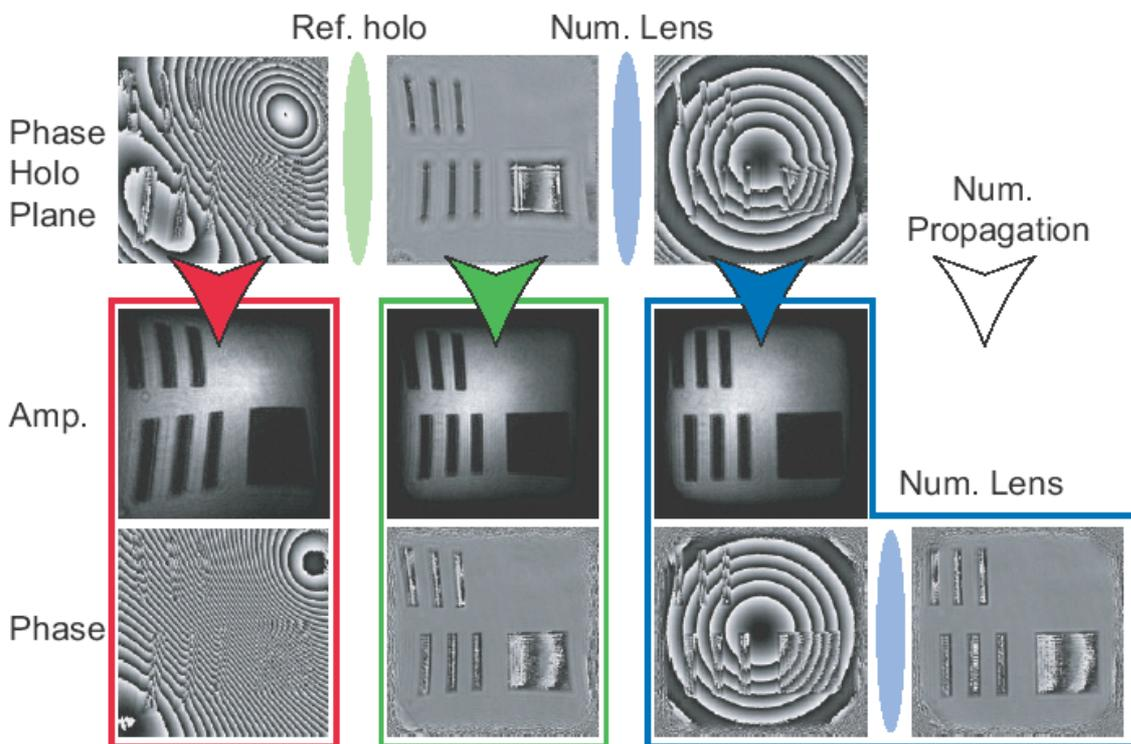
**Figure 2:** Complete numerical compensation for image distortion and phase aberration induced by a lens ball used as MO. In red, the reconstruction without compensation; in green after the reference hologram method correction; and in blue the manual compensation for residual image distortion.
