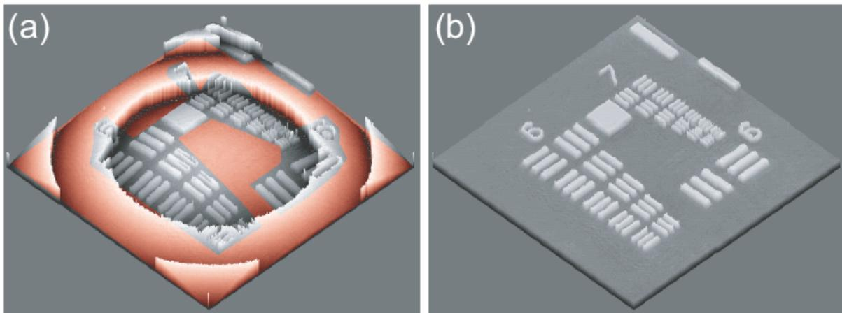
**Figure 1:** Compensation for phase aberrations by computation of the polynomial coefficients of the numerical lens. 3D representations of the phase images of a USAF test target (a) before and (b) after aberrations compensation (assumed flat areas in red).
