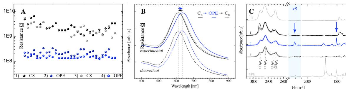
**Fig.2:** **A.** Electrical resistance of 30 devices, switching successively from unlinked (high R) to OPE-linked (low R); **B.** Visible absorption spectra of a device unlinked (black), OPE-linked (blue) and unlinked again (grey dashed). **C.** FTIR spectra for the same sequence, with the references (light grey) for free alkanethiols and free OPE molecules.
