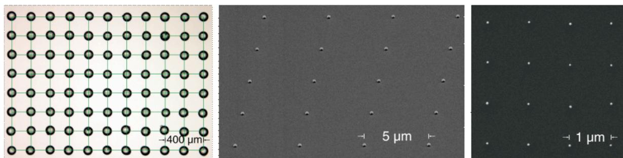
**Figure 3.** Spaced, regular particle arrays. From left to right, 100- $\mu\text{m}$  glass beads on glass, 500-nm polystyrene spheres on silicon oxide and 60-nm gold crystals on silicon [1].
