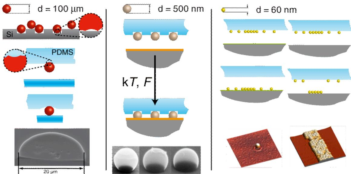
**Figure 2.** Adhesion-based handling of particles. Depending on the particle diameter and material, adhesion cascades to transfer particles from one surface to another can be created by exploiting hard versus soft contacts and adhesion layers (100  $\mu\text{m}$  glass beads), softening of the particles and thus increase of interfacial area (500 nm polystyrene latex) or particle interactions and adhesion layers (60 nm gold nanocrystals).
