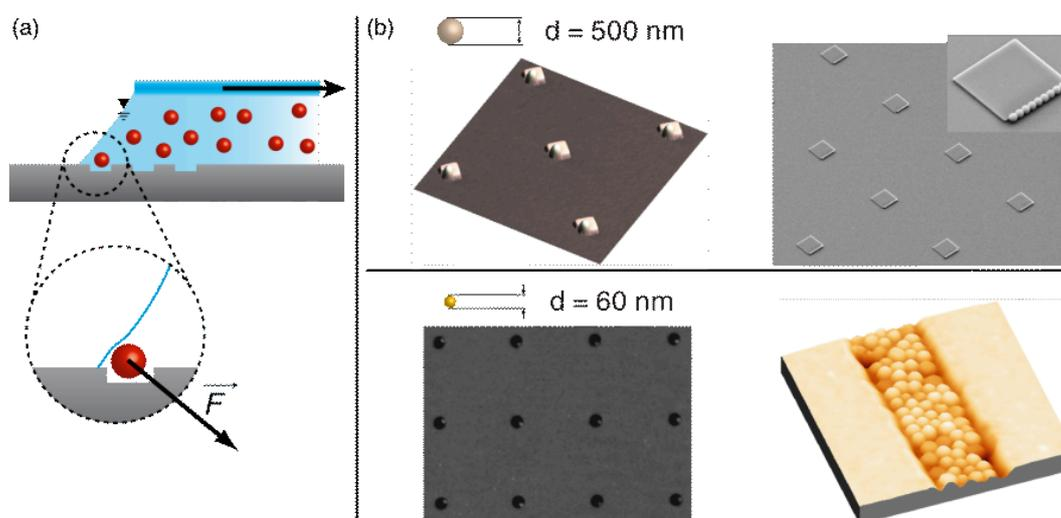
**Figure 1.** Capillary assembly of small particles. (a) The meniscus of a colloidal suspension is moved over a patterned substrate. A contact angle of about  $60^\circ$  prevents unspecific deposition, while appropriately-shaped binding sites capture particles at predefined locations. (b) Particles assembled in different geometries.
