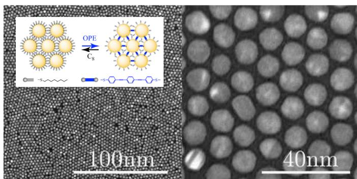
**Fig.1:** Self-assembled monolayer of functionalised gold nanoparticles (magnifications); inset: schematics of the reversible place-exchange.
