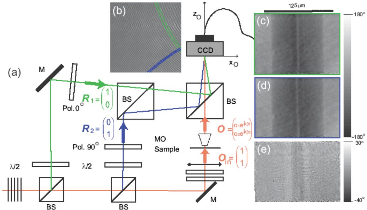
**Figure 3:** Polarization imaging by DHM. (a) Setup, (b) hologram, (c-d) reconstructed phase images from interference of object wave O with the orthogonal polarized reference waves R1 and R2; and (e) phase difference image revealing internal stress in an optical fiber.
