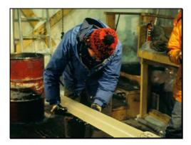
This figure shows one of these ice cores to be analysed, 10 cm in diameter and in average about 2.5 m long per run.
