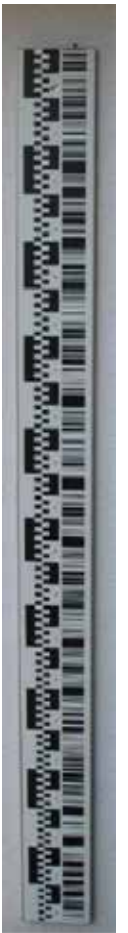
Figure 2: Level Rod (Classical scaling, left) and Leica barcode (right)
