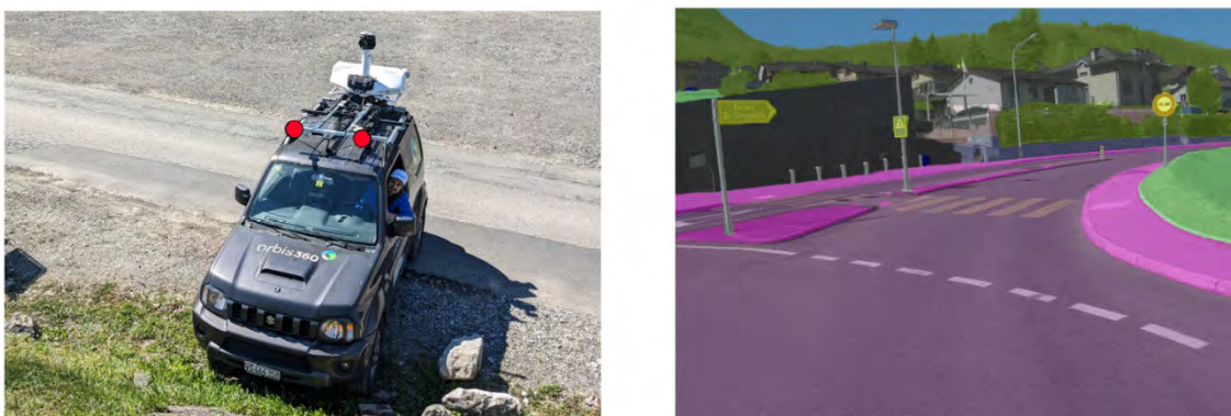
Figure 1. Left: stereo pair coupled in red with RTK positioning placed on a car (Orbis 360), right: inference using the pre-trained model (Chen et al., 2022)
