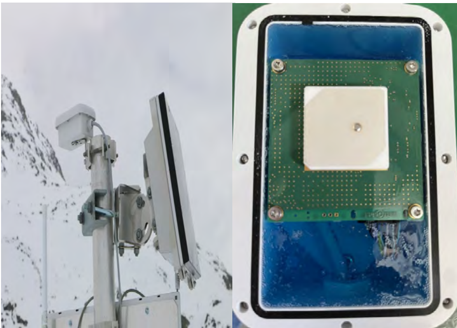
Figure 2 Left: Astronode S+ satellite transceiver at the test station connected to the monitoring system by SensAlpin GmbH; Right: the Astronode S+ in a sealed housing with sealing compound (source: SensAlpin GmbH)
