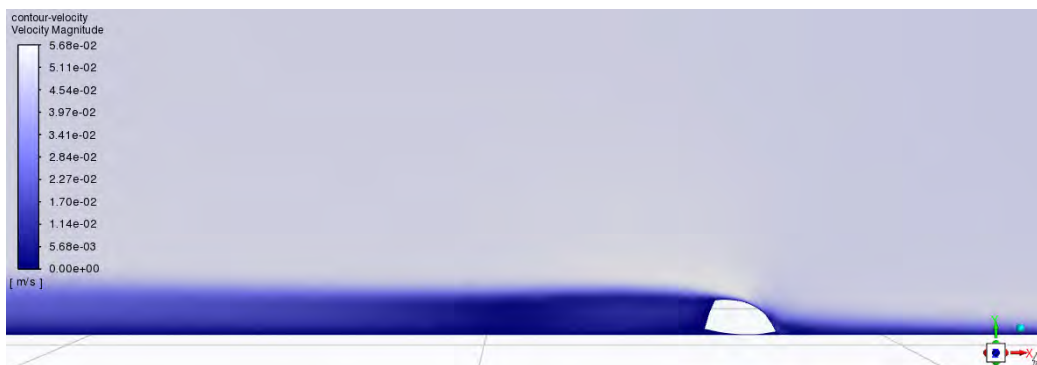
Figure 1. Example simulation of water flow around a trilobite cephalon, produced using Ansys Fluent.
