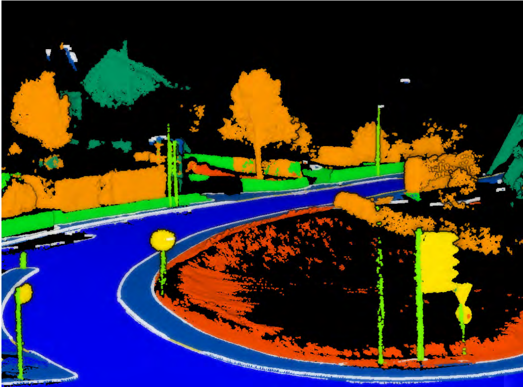
Figure 2. Reprojection of the classification in the 3D model and highlighting of white sidewalks and green curb cut by extraction in the geometry
