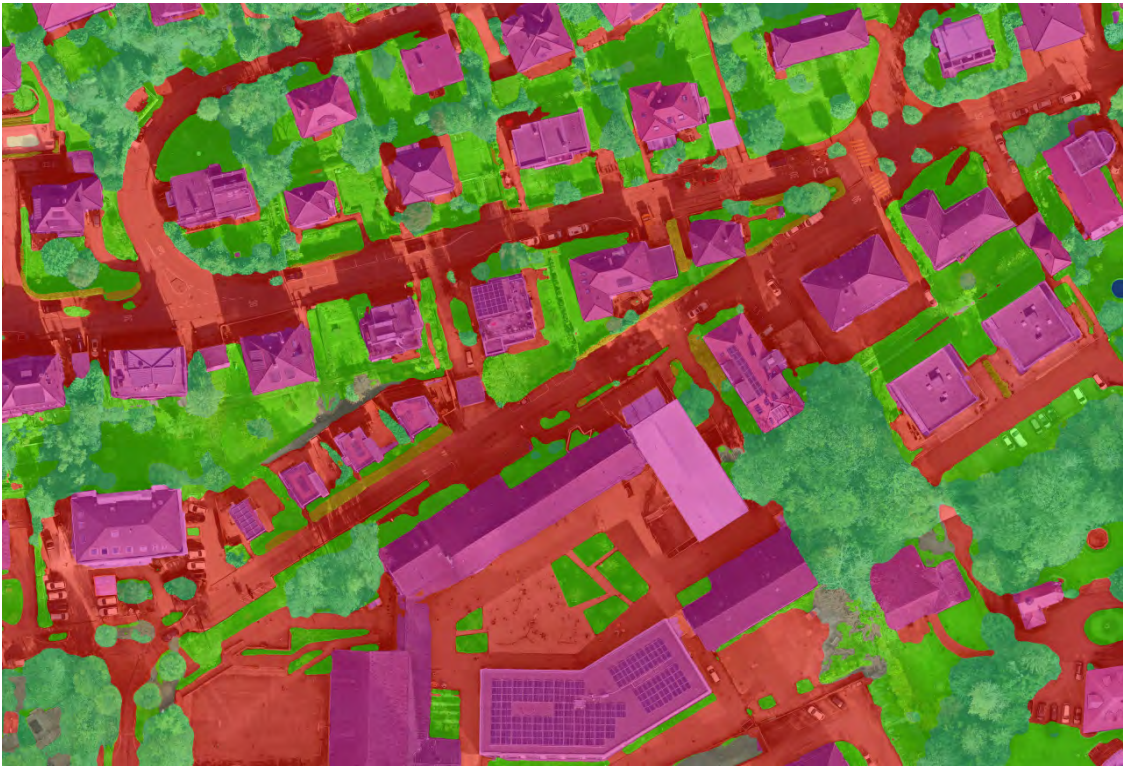
Figure 2. Result of the AI trained during the challenge on an ortho image of Friburg with a ground pixel of 10 cm.
