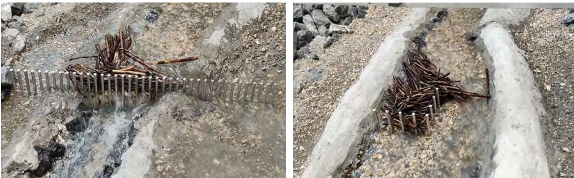
Figure 3. Two different rack configurations to retain wood debris
