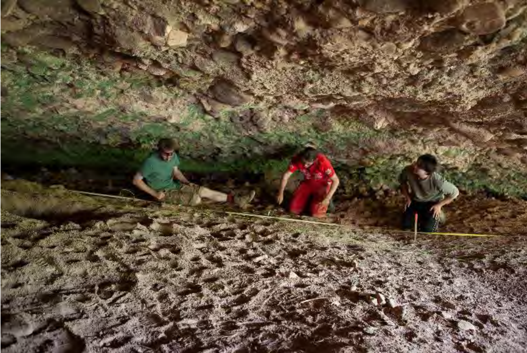
Figure 2. Setting up electrodes for the ERT lines. (Fabio Wegmüller)
