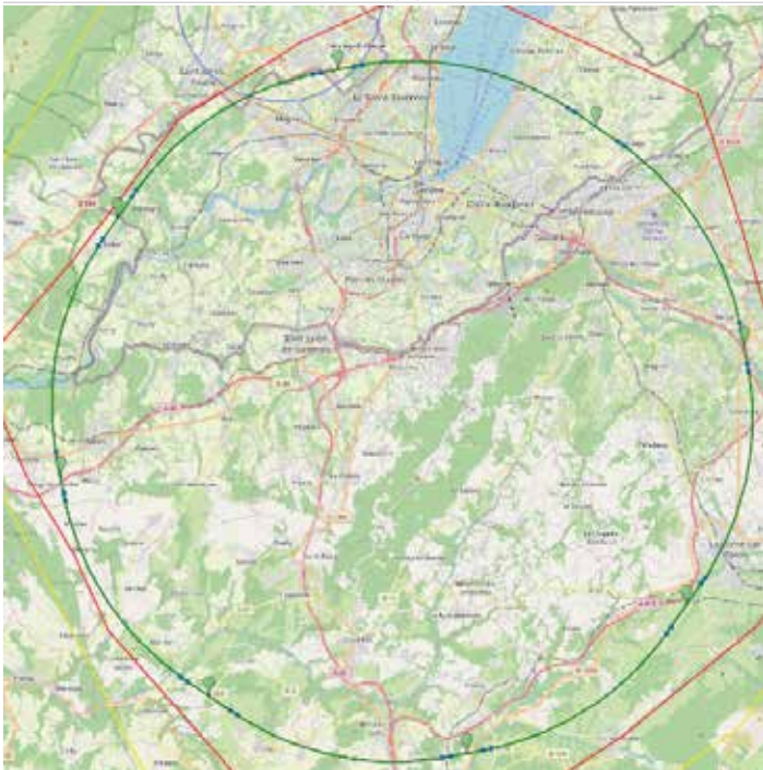
Fig. 1: Schematic views of the FCC-ee accelerator (90.7 km long) and its indicative geographical implantation. The scheme shows in green the booster (not to scale), where the electron and positron bunches are accelerated, and in blue the storage rings, where the two beams circulate in opposite direction in separate beampipes except in the four interaction points where collisions take place. Courtesy of M. Benedikt, J. Gutleber and V. Mertens (CERN).
