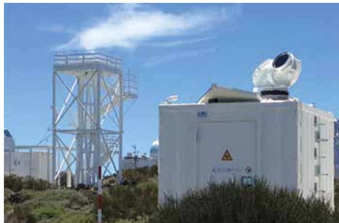
Fig. 6: Ground station on Tenerife for up- and down link to satellites using laser light as data carrier. Image: GA-Synopta GmbH.
