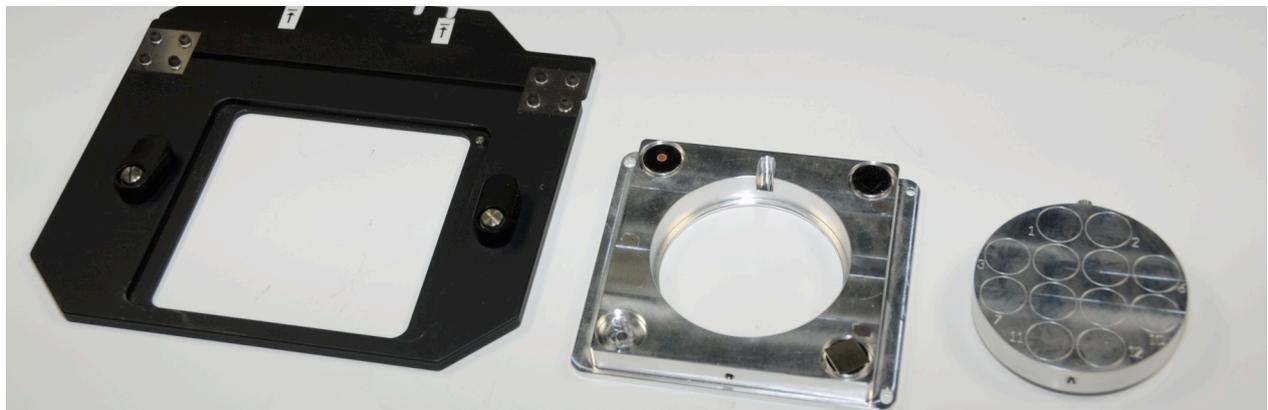
**Fig. 2:** Holder system consisting of an LM adapter, a holder frame with markers and a core disc with samples attached to the surface. In the corner of the holder, stub positions are available for reference samples.
