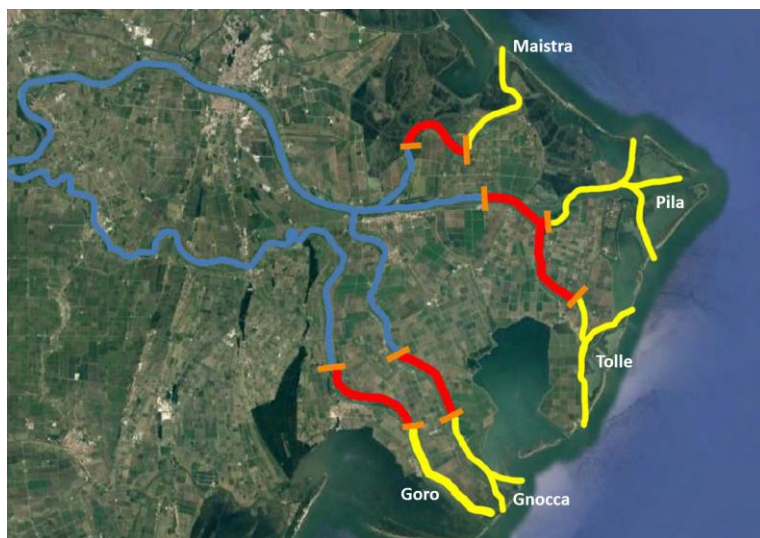
Figure 9: Sea water intrusion distance in km at mid-April 2022 compared to the values corresponding to the reference critical threshold of 450 m 3 /s river discharge (upper) and location of river branches (lower). Source: Permanent Observatory on water use - Po River District Basin Authority.
