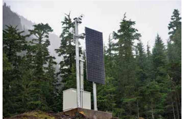
Avalanche radar with high-resolution camera with autonomous power supply and redundant radio connection for communications at Bear Pass, British Columbia, Canada.
