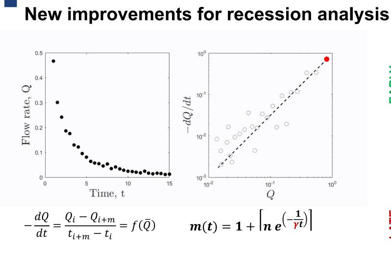
Derivative estimated using the local slope coefficient of a least-squares linear regression function over  $[t_i, t_{i+m}]$ ; Direct linear fitting and residual coefficient (R2) from the local linear fit as weight vector.
