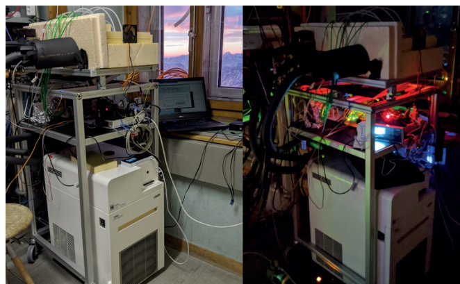
Figure 2: An image of the automated Horizontal Ice Nucleation Chamber (HINC-Auto) sampling aerosol particles directly from ambient air at the Sphinx Observatory, Jungfrauoch.
