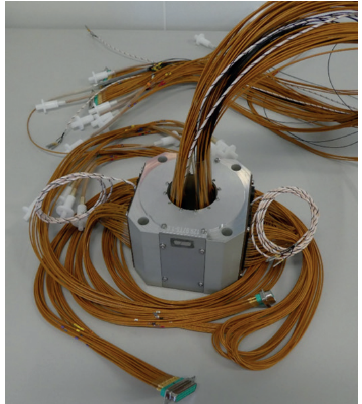
Figure 6: Picture of the BBM implementing the passively-biased LDs [source: Beyond Gravity].
