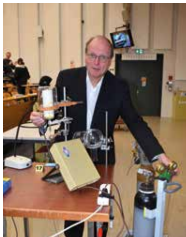
Fig 2: Jean-Philippe Ansermet demonstrating the Dufour effect, where a Helium concentration gradient in a porous wall induces a local temperature change at the thermocouple.
