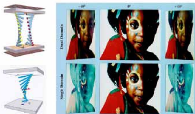
Fig.9: Single- and dual-domain photo-aligned TFT-addressed TN-LCD and corresponding nematic director configurations in the on-state; c.f. the much enhanced field of view of the dual domain configuration.
