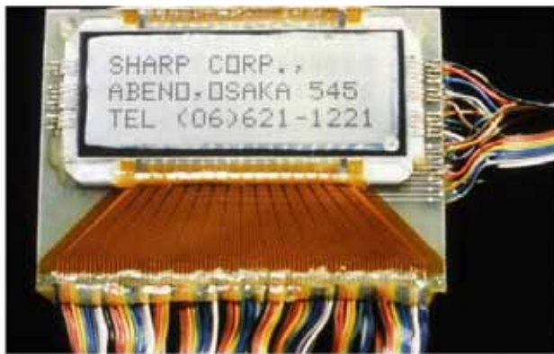
Fig.4: Time-multiplexed addressing scheme of the line and column electrodes of a TN-LCD (top). Time-multiplexed TN-LCD with 1200 pixels but only 96 connections (~1980).
