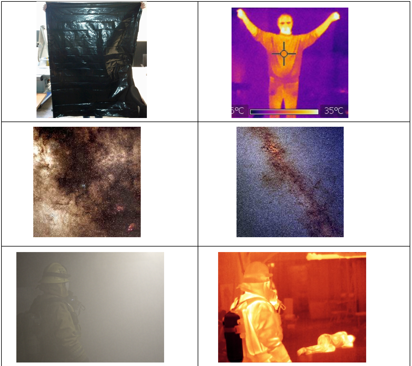
Fig. 1. Looking behind the curtain: Infrared images from man to milky way, and back to everyday life 1) Top: Behind a plastic “curtain” (PE): person in visual range invisible (left), in infrared range visible (right). 2) Middle: Behind the dust “curtain” (interstellar dust): galactic centre in visual range invisible (left), in infrared range visible (right). 3) Bottom : Behind the smoke “curtain”: Firefighter searching for a victim: invisible in the visual range (left), visible in infrared range (right).
