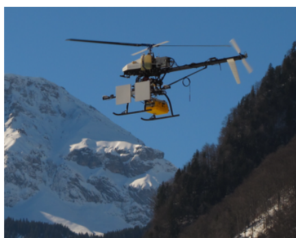
Figure 1: GAMMA L-band SAR on Aeroscout's VTOL UAV Scout B1-100, equipped with a Honeywell HGuide n580 INS/GNSS navigation system, at the test site Wolfenschiessen, Switzerland.
