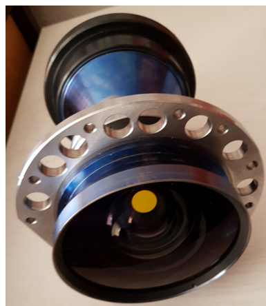
Figure 2: Wide angle lens. The yellow spot indicates the entrance pupil at large field angle
