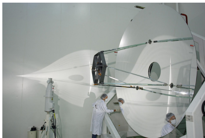
Figure 3: Herschel telescope with EP diameter of 3 m. On the left a Leica laser tracker for interferometric testing
