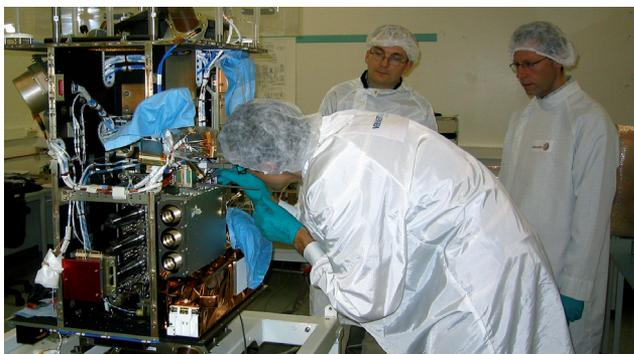
*Integration of LYRA on the spacecraft PROBA 2 on March 5, 2007 at the Belgian firm Verhaert Space. The person on the right is Silvio Koller, LYRA instrument engineer at PMOD/WRC, responsible for all manufacturing aspects of the hardware and electronics.*
