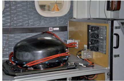
*Support grid and scintillating bars mounted in one module target*
