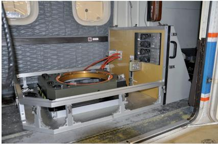
*APEX Thermal Control Unit in Dornier DO-228 aircraft including Leica stabilizing platform*
