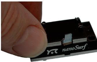
Assembled AFM scanner with mounted silicon sensor chip
