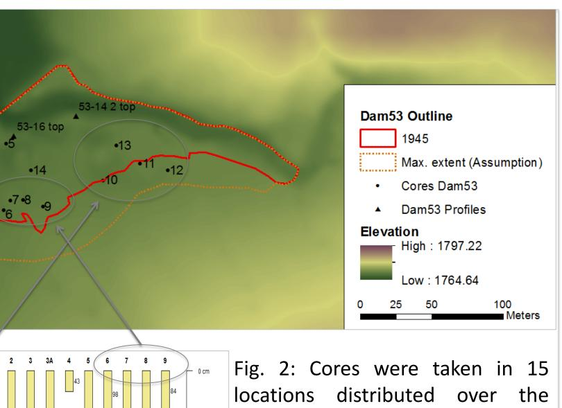
former reservoir area and are still to be analysed for physicochemical parameters of sediment layers. The depth of each core is shown in the figure. Lower depth for cores 6 to 12 indicate an asymmetric cross profile shape of the reservoir. The short column of core 4 is most likely explained by a rock that was
