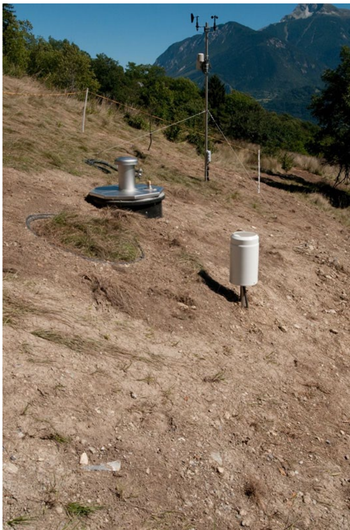
Figure 2. Hillside Lysimeter with exte tensiometer and weather station, Lens-Chermignon, August 2010.
