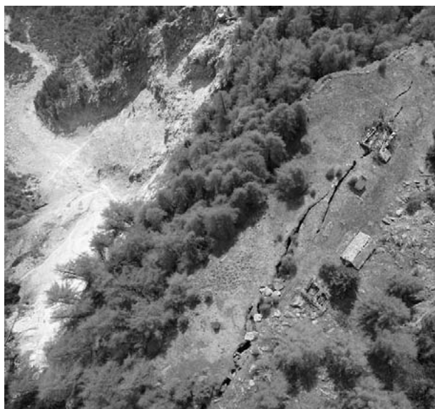
Figure 1. High resolution aerial image of Alp di Rosciro: The large tension cracks behind the main scarp can be clearly identified.
