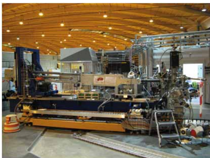
Figure 4: RIXS endstation at the ADRESS beamline of the SLS consisting of the analysis chamber (on the right), SAXES spectrometer and rotatable girder platform.
