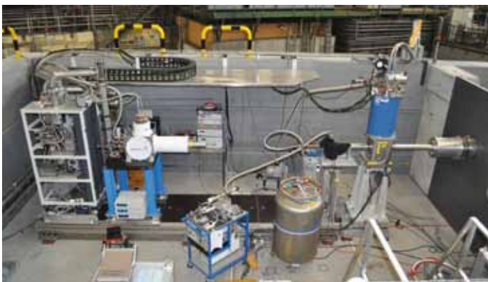
Figure 2: The new instrument for high-field \mu SR at PSI. The 9.5 T magnet is on the right (blue). On the left the dilution refrigerator with gas handling system is visible (white), cooling samples to temperatures below 20 mT.
