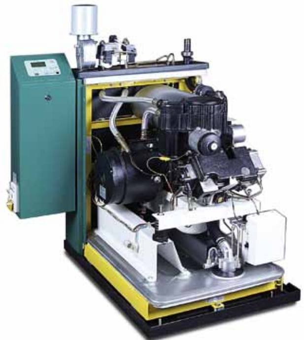
Fig.2: Mini Cogeneration machine of 5.3 kW el rated power [5]. Above the cylinder head ("SACHS") one sees the heat exchanger for the exhaust gas (black), the water cooled generator is at the left side.
