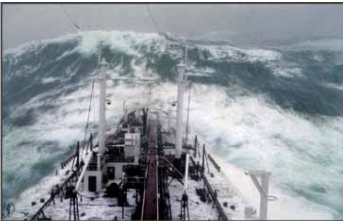
Figure 1. A wall of water approaches the Stolt Surf in October 1977. The chemical tanker encountered a wave of at least 22 m, much higher than the significant wave height estimated to 10 m. Photo credit: Karsten Petersen, www.global-mariner.com
