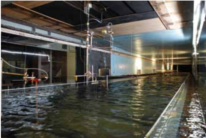
Figure 4. Wind-wave facility at Pythéas-IRPHE in Marseille (France). Photo credit: Arthur Lemoine. The tank is 40 m long, 3 m wide and 0.9 m deep. It is equipped with a recirculating wind tunnel that can generate wind speeds between 1 and 14 m/s.
