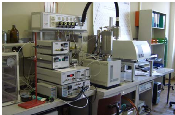
Figure 3: Pulse TA coupled to a mass spectrometer for studies on in-situ gas solid reactions.
