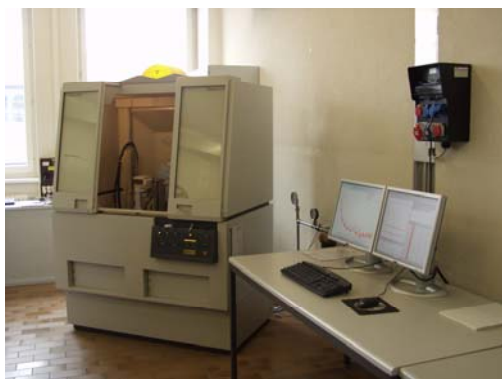
Figure 2: X-ray diffractometer. Calculated (red) and observed XRD pattern of \text{LaTiO}_2\text{N} crystallized in perovskite-type pseudo-cubic unit cell [Logvinovich, D., Börger, A., Döbeli, M., Ebbinghaus, S.G., Reller, A. and Weidenkaff, A, Synthesis and physical chemical properties of Ca substituted \text{LaTiO}_2\text{N} , Progr. in Solid State Chem. , in press.]
