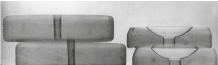
Fig. 23: Nd:YAG drilled holes (diam. 50 \mu\text{m} ) in 0.3 mm thick ruby discs (diam. 10 mm) and finished watch bearings [100].
