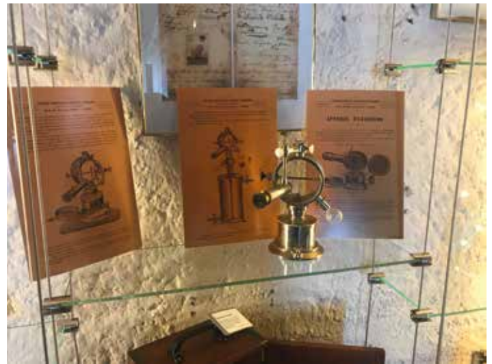
Figure 5: Electrometer from Albert Gockel's legacy, on loan from Uni Fribourg. From the Société Centrale de Produits Chimiques , 44 Rue des Ecoles Paris, ca. 1910. In the back, reprint from the original vending catalogue, featuring the device.
