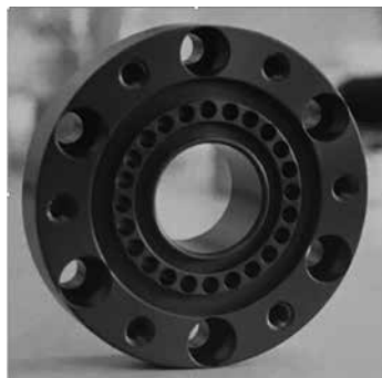
Fig. 13: Ar-ion laser discharge tube segment with 32 mm inner diameter [59].
