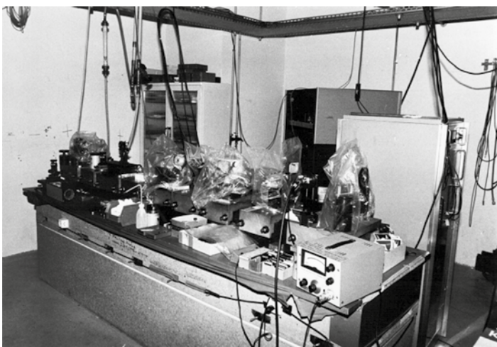
Fig. 11: Nd:glass amplifier table. Two 20 mm diameter rods pumped by helical flashlamps (KORAD Laser Systems) boosted the pulse energy to \sim 1 J [29].
