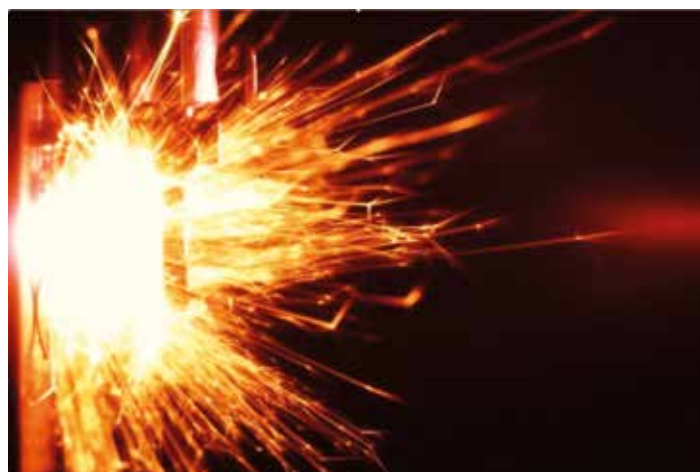
Fig. 4: Impact of ruby laser pulse on razor blade [7]
