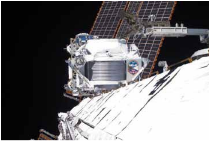
Figure 1: From its vantage point about 400 km above the Earth, the Alpha Magnetic Spectrometer (AMS) collects data from primordial cosmic rays that traverse the detector.
