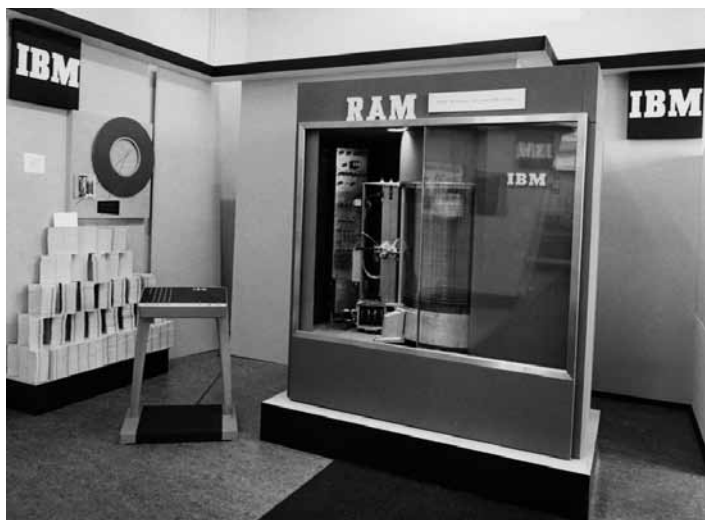
Fig. 3. Introduced in 1956, the IBM 305 RAMAC (Random Access Memory Accounting System) was an electronic general purpose data-processing machine that maintained business records on a real-time basis. The 305 RAMAC was one of the last vacuum tube systems designed by IBM, and more than 1000 of them were built before production ended in 1961.
