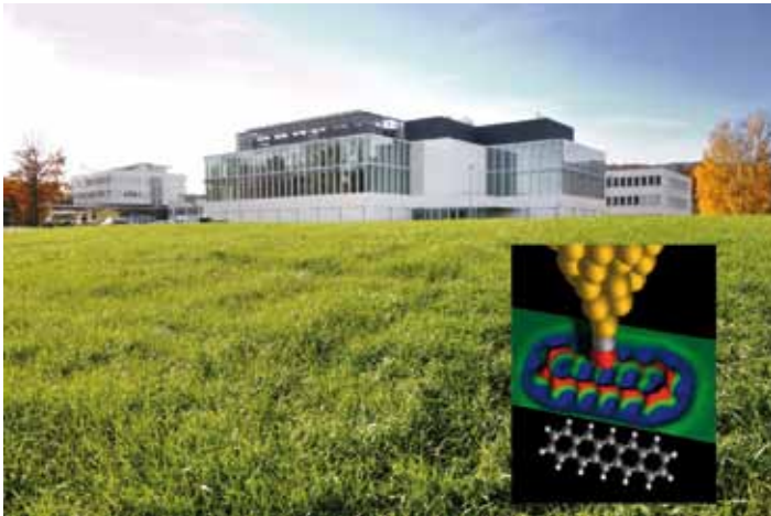
Fig. 4. The newly built Binnig and Rohrer Nanotechnology Center and as inset an example of the complete atomic structure of a pentacene molecule resolved by AFM [2]. The extreme resolution of the C, H atoms and chemical bonds is achieved by the CO molecule attached to the tip.
