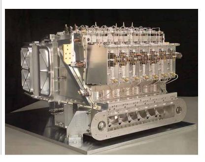
Common Optics Assembly of HIFI on the Herschel Space Observatory, an ESA space craft that operated at the Lagrangian Point L2, 1.5 million km from Earth. The mechanical structure and components were produced by RUAG Wallisellen.
