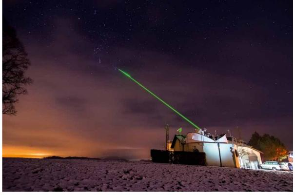
Laser beam transmitted from the 1-meter Zimmerwald Laser and Astrometry Telescope (ZIMLAT) to measure high accuracy distances of artificial satellites.
