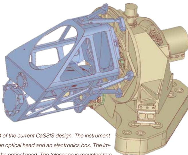
A CAD/CAM of the current CaSSIS design. The instrument comprises an optical head and an electronics box. The image shows the optical head. The telescope is mounted to a rotation drive which allows production of stereo images by rotating the telescope through 180 deg to produce a stereo convergence angle of 22 deg.
