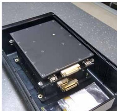
*Flight Model of the Filter Wheel Electronics (FWE).*
