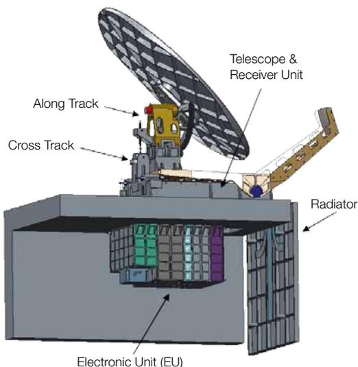
*Submillimeter Wave Instrument (SWI) for the ESA mission JUICE to Jupiter and its icy moons. The instrument consists of a radiometer/spectrometer operating between 530 and 630 GHz and a telescope with 30 cm aperture.*
