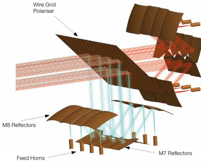
*Focal Plane Array (FPA) optics for the multi-beam limb sounder STEAMR on the ESA Earth Explorer Mission PREMIER. The ray tracing model shows how the signal path of fourteen 340GHz receivers is combined using a polarized beam splitter and a set of interleaved facet reflectors.*
