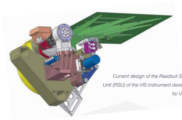
Current design of the Readout Shutter Unit (RSU) of the VIS instrument developed by UNIGE.
