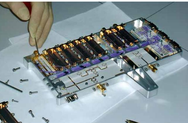
The frequency amplification unit, including low-noise and low-power amplifiers (InP HEMTs), for the HIFI instrument on the Herschel Space Observatory. The unit was designed and constructed by the Laboratory for Electromagnetic Fields and Microwave at ETH Zurich. The figure shows the qualification model. The flight model was produced by RUAG Aerospace Oerlikon and Baumer Electronics, Frauenfeld.
