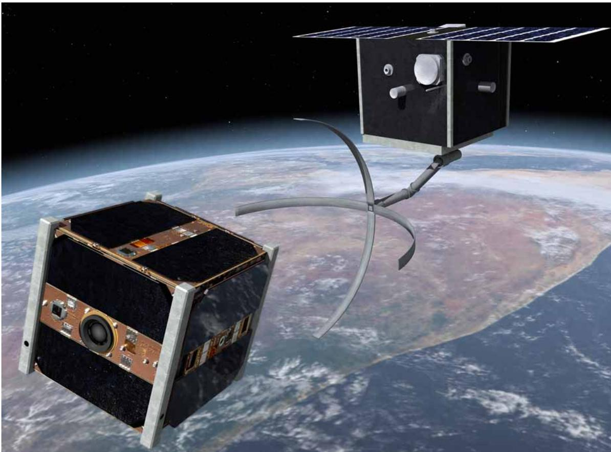
*At close quarters CleanSpace One will very carefully perform the "Hug-Me" maneuver to catch the slowly rotating debris. These operations, may be partially done autonomously by CleanSpace One. The compliant grabbing system will utilize a MEMS based system to deploy and then wrap around the object in space. It will be inspired from nature's catching behaviors.*
