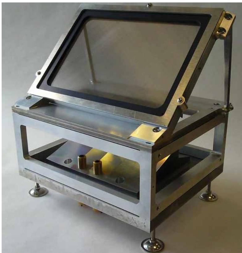
A breadboard model of the FPA has been manufactured and characterized by near field antenna measurements.
