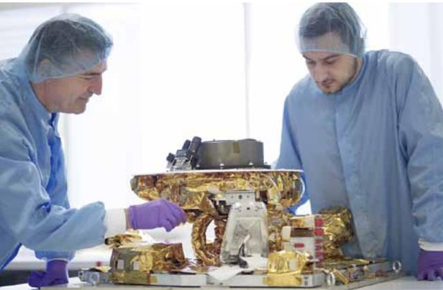
*Integration of an alignment-mechanism. used for the electrical power transmission of a satellite.*
