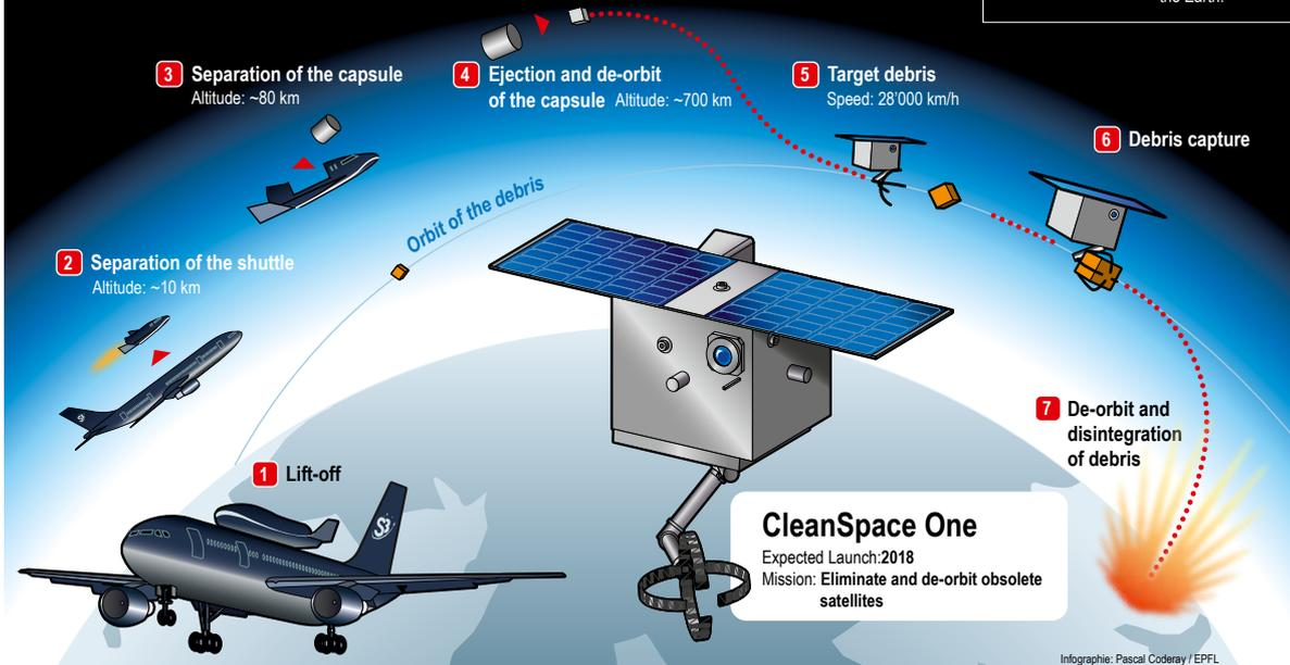
*CleanSpace One will de-orbit space junk: After ejection from the launch vehicle, propulsion maneuvers will be performed to reach SwissCube's orbit. These maneuvers will rely on ground radar observations of the debris and the onboard GPS on CleanSpace One. Approach maneuvers will be performed to further reduce the distance to a few meters. These maneuvers will rely on optical, radar or lidar technologies.*
