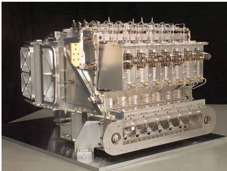
Common Optics Assembly of HIFI on the Herschel Space Observatory, an ESA space craft that operated at the Lagrangian Point L2, 1.5 million km from Earth. The mechanical structure and components were produced by RUAG Wallisellen.
