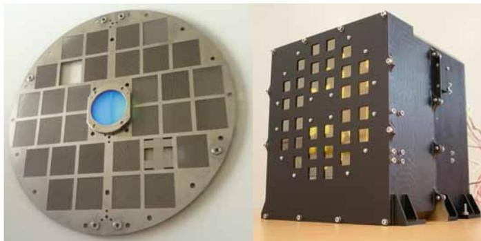
Structural Thermal Model of one of the two STIX tungsten grids with the blueish aspect lens (left) and the Detector Electronics Module with the 32 openings behind each an X-ray detectors is placed (right). The two grids are placed in front of the X-ray detectors to produce a Moire pattern on the X-ray detectors so that the imaging information is stored in the relative count rate of the different pixles (i.e. each detector provides a Fourier component).
