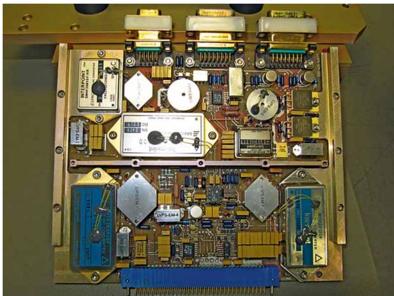
Engineering Model (EM) of the Low Voltage Power Supply (LVPS) for the SPICE instrument built at PMOD/WRC. The EM of the LVPS has been integrated into the SPICE Electronic Box and undergone thermal and vibrational tests. The functional, electronic and magnetic cleanliness tests of SPICE at full instrument level are currently being carried out at RAL.
