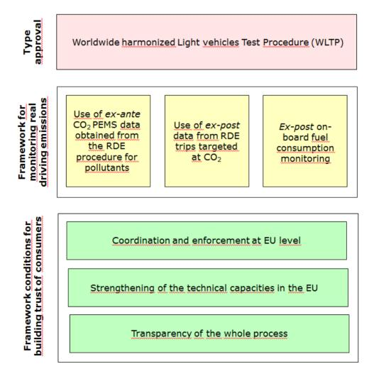
*Figure 4: Necessary elements to close the gap between laboratory measurements and real driving emissions*
