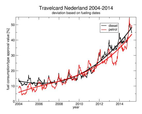
Figure 3: Development of real-world fuel consumption versus type approval values according to Travelcard Nederland
