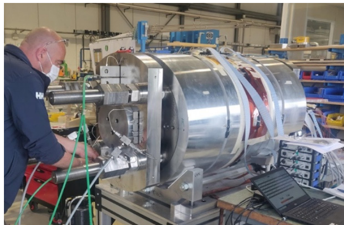
Figure 5: The RMM1 single-aperture dipole, designed and built at CERN, in the final steps of magnet assembly. The magnet reached ~17 T maximum field and 16 T stable operational field.
