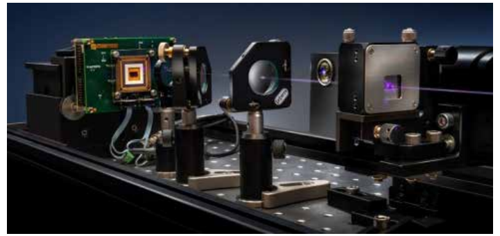
A setup used for quantum ghost imaging, where a special crystal is used to generate entangled photon pairs of different wavelengths from laser light (Image: Fraunhofer IOSB)
