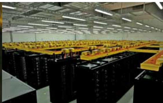
Energy Efficiency by Warm Water cooling - Super-MUC Petascale Cluster at the Leibniz Supercomputing Center. See p. 12. Photo: ©: IBM Research - Zurich
