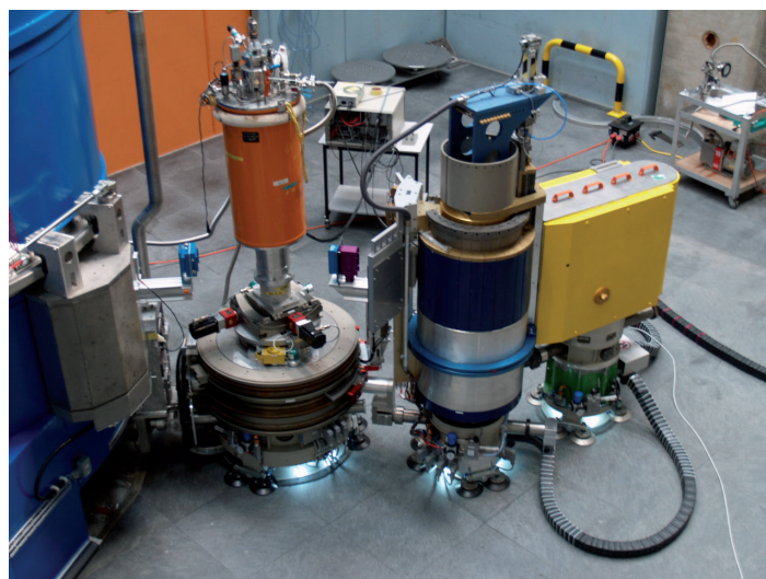
Figure 1: The new thermal triple-axis spectrometer EIGER at SINQ.
