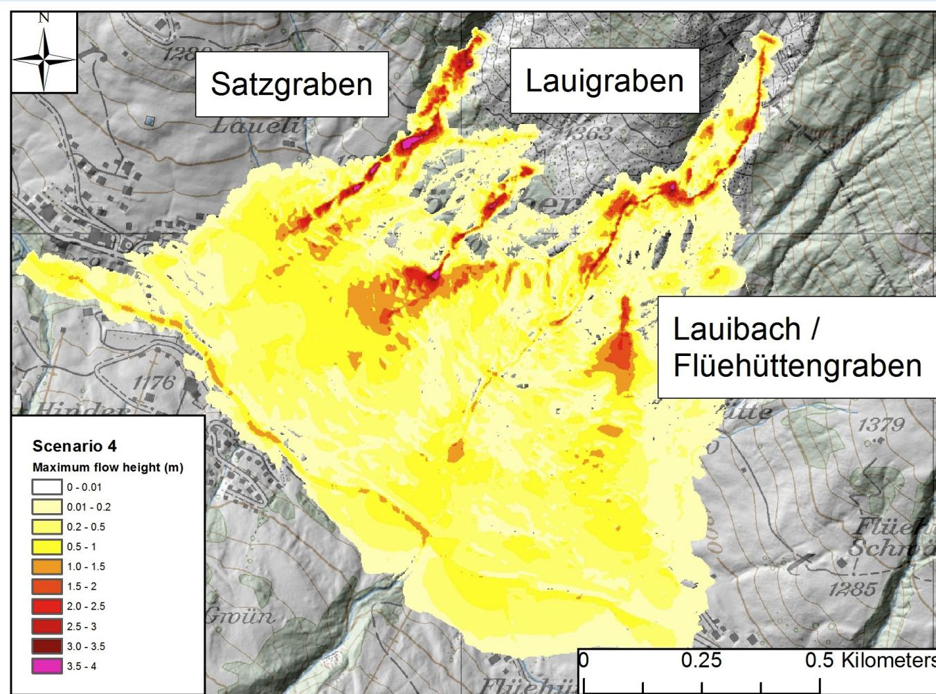
*Data source of map and digital terrain model: Swisstopo 2012, 2010; modelled with RAMMS debris flow.*
