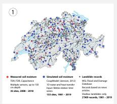
All available continuous soil moisture measurements in Switzerland were gathered and soil moisture was simulated at meteorological sites. Soil moisture was normalized ('saturation') and profile mean and SD was calculated. Landslide information was taken from the Swiss Flood and Landslide database (WSL).
