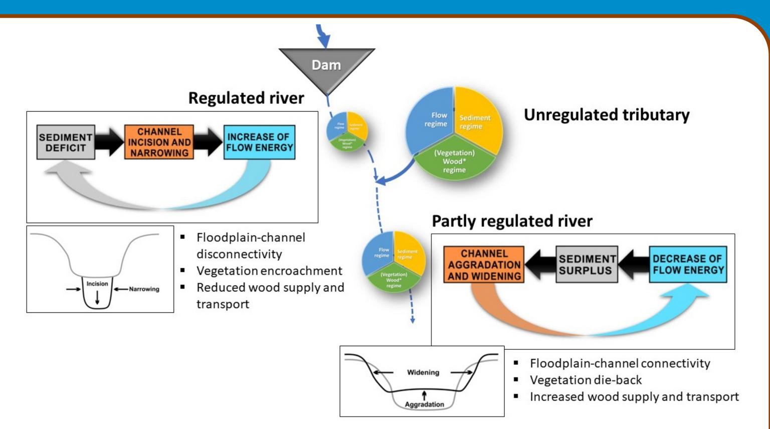
The riverregulated by a dam results in narrowing and incision processes due to the flow and sediment deficit, but if an unregulated tributary joins the regulated river, as in the case of the Spöl River, the downstream segment becomes only partly regulated and is characterized by different processes.
