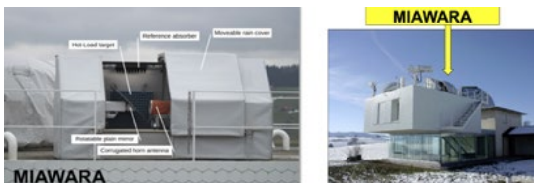
Figure 1. The observatory for water vapor at Zimmerwald and the Middle Atmospheric Water Vapor Radiometer (MIAWARA).
