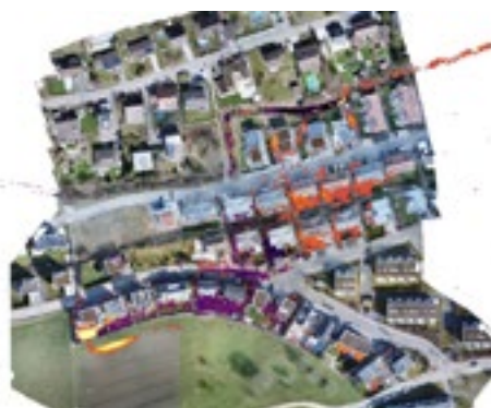
Figure 2 Clipping simulation result (difference plot depth between LIDAR mapping and terrain mapping by a drone)
