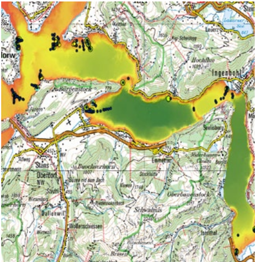
Figure 1. Map of measured CPTu profiles (dark blue circles), retrieved sediment cores (green circles), OBS single station (blue triangles) and OBS array (yellow circles) measurements.
