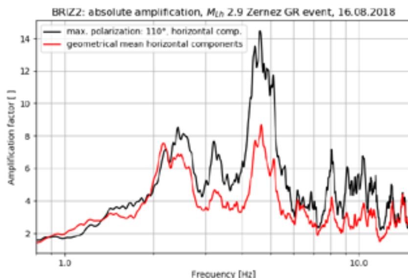
Figure 1. Absolute amplification spectrum of the station BRIZ2, installed on the rock slope instability Brienz / Brinzauls. The input data is the M_{Lh} 2.9 earthquake in Zerne (40 km epicentral distance).
