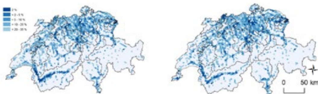
Figure 1. Spatial distribution of Switzerland's most flood exposed building values, estimated by (left) a straight forward model based on flooded area and land use and (right) a sophisticated model based on individual building parameters including volume. Blue indicates for both models the upper 35% of flood exposed building values.
