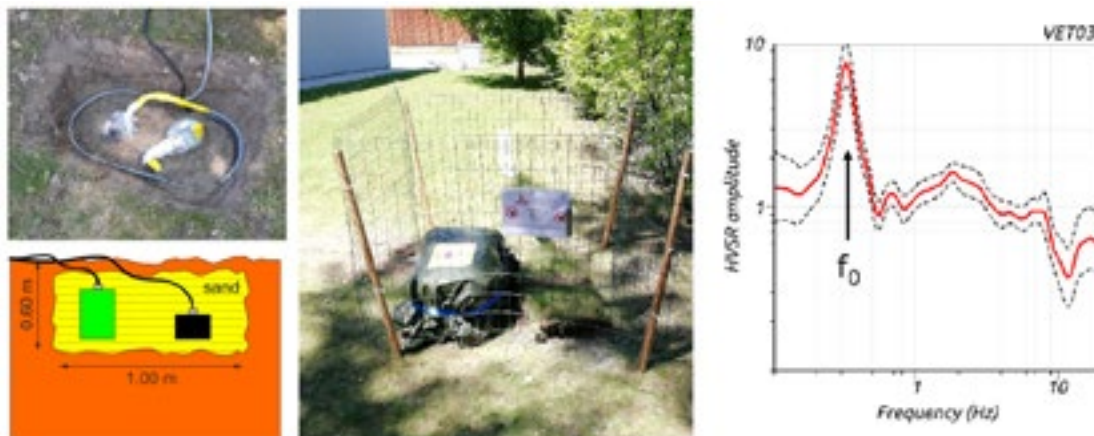
Figure 2. Sensor installation at site VET03, measured HVSR curve and deduced fundamental resonance frequency ( f_0 ) for the site.
