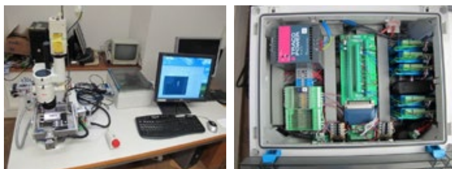
Figure 1. New AMOR 2 (22 August 2018). Left, Motorized 4-axis tilting stage combined with a binocular microscope, digital camera, motorzoom and motorized magnification changer. Microfossils placed in the Plummer cell can be automatically positioned under the microscope and oriented, focused, and imaged. Right side: Box containing motion controllers and electronics. The robot is operated via customized AMOR4 software written in LabView 14. In contrast to the earlier version, AMOR2 has additional functions for microfossil orientation and does no longer need a frame grabber. AMOR2 would not have been possible without the help of Daniel Binggeli (FHNW) and voluntary worker at NMB, Prof. em. Jean Eisenecker (FHNW).
