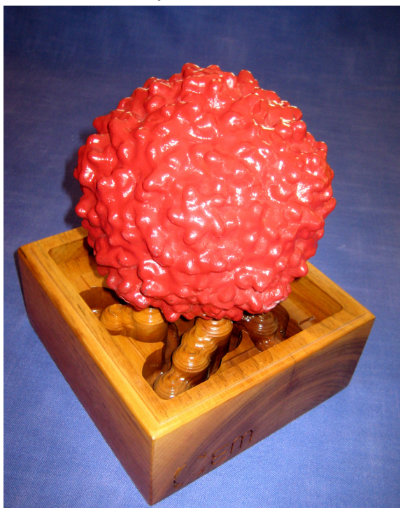
Figure 1: Rapid prototyping was used to create a 20cm diameter plastic machete of the polio virus capsid (2.2Å resolution, Hogle Laboratory, Harvard Medical School) for the 2005 Smithsonian Exhibition commemorating the 50 th anniversary of the polio vaccine with complementary walnut base
