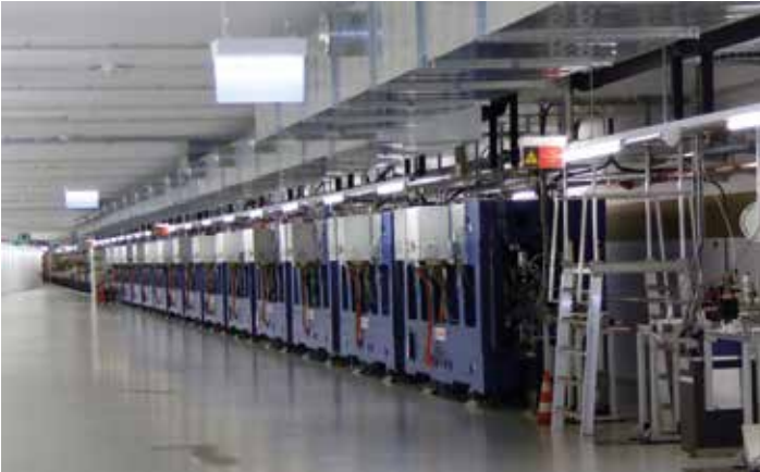
Fig. 4: The SwissFEL undulator magnets
