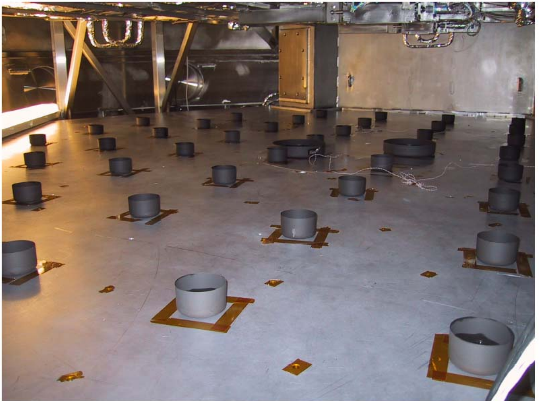
liquid mirrors are aligned on optical bench inside the chamber
