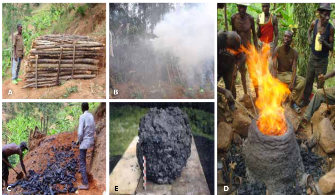
Figure 3: Steps involved in charcoal and iron production: (A) Stacked wooden logs; (B) Slow combustion of the wood; (C) Charcoal produced by combustion; (D) Iron ore reduction using a traditional furnace; (E) Spongy iron (bloom). 5
