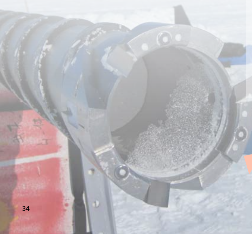
Figure 2: Cutting end of the ice-core drill. The three blades are the cutters that cut around the ice core, which you can see just inside the hollow section of the drill.
