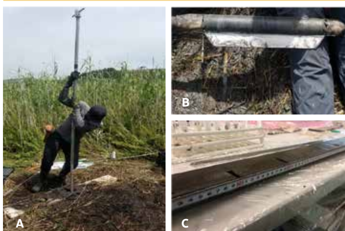
Figure 4: (A) This researcher is using a Russian corer to bore into the fen and recover the layered sediments (core); (B) The recovered core with its layers visible; (C) How we slice the core into chunks before processing (University of Melbourne Palaeoecology-Palaeoclimatology).
