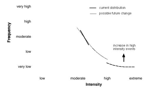
Fig. 1: Distribution curve for daily precipitation events. Intensity is based on a logarithmic scale. The broken line represents the part of the curve for which it is not possible to make statistically well founded statements regarding trends in frequency based on current data.
