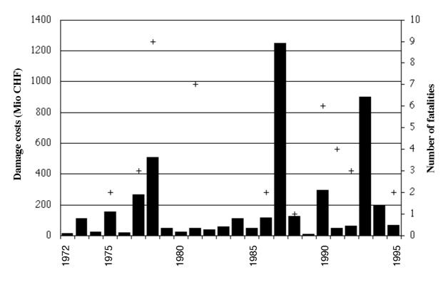
Fig. 4: Annual damage (bars) and fatalities (+) caused by high-water events in Switzerland (Röthlisberger, 1998; not corrected for inflation)
