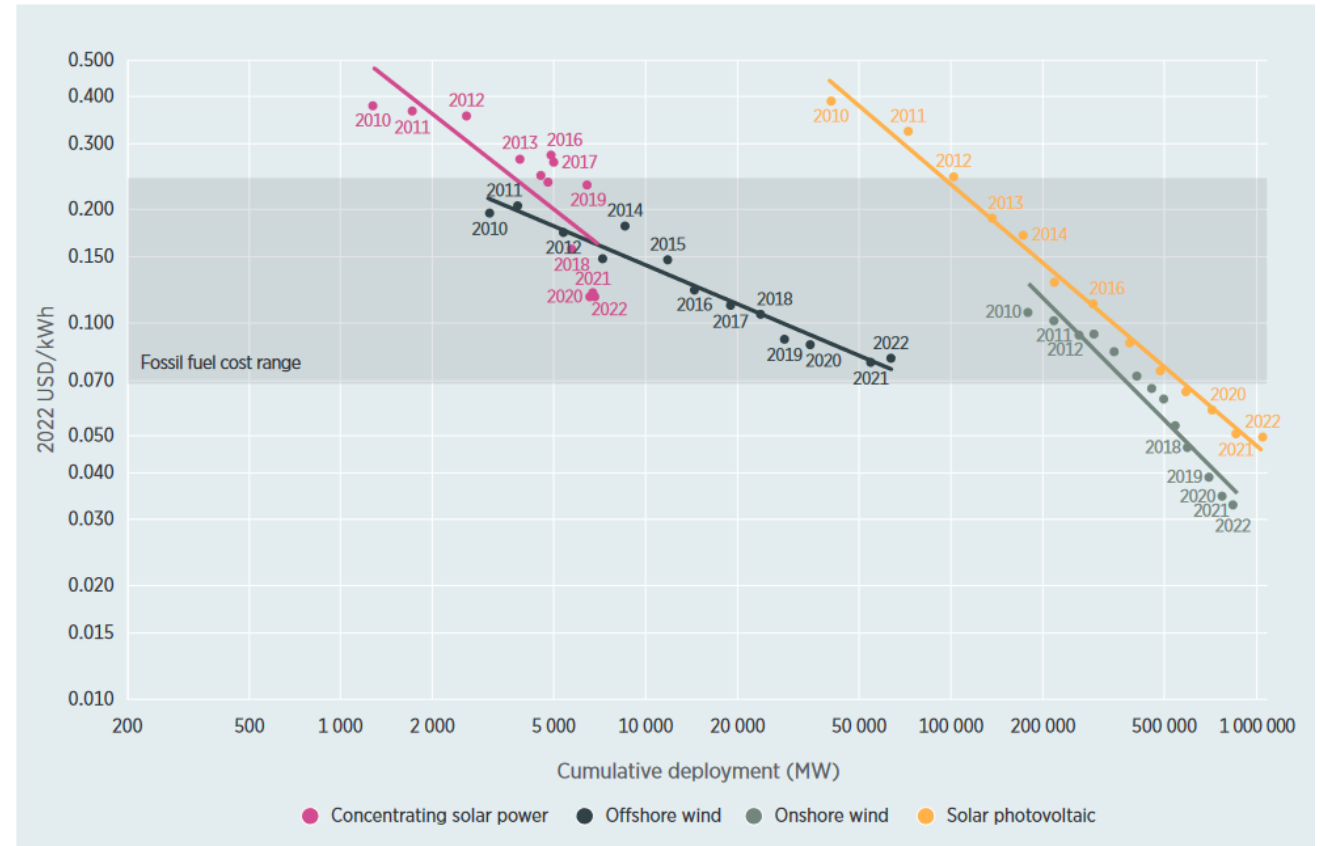
Global weighted average LCOE learning curve trends for solar PV, CSP, onshore and offshore wind, 2010 – 2022 [1]
